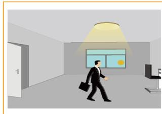
The lamp switches on when ambient light is lower than preset illumination level and motion is detected.
